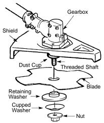
**NOTE:** Make sure all parts are in place as il-lustrated, and the blade is sandwiched between the dust cup and the retaining washer. There should be no space between the blade and the
